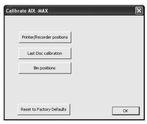
Last Disc calibration and Bin positions will only be necessary if the Autoloader is having trouble picking from the bins. Follow the on-screen prompts to calibrate the bins.
